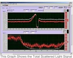
Resulting from a Particle Passing Through the Laser Beam. Note the System Triggering at t=0.
