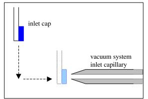
Figure 4. Schematic diagram of the functionality of the inlet cap system.
