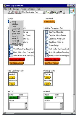
Figure 3. Front panel of the Inlet Cap Driver.vi.
