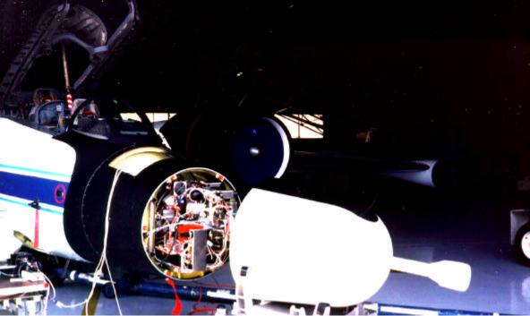
Figure 1. The PALMS instrument loaded into the nose of the WB-57 aircraft.
