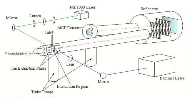
Figure 2. Schematic of the PALMS instrument.
