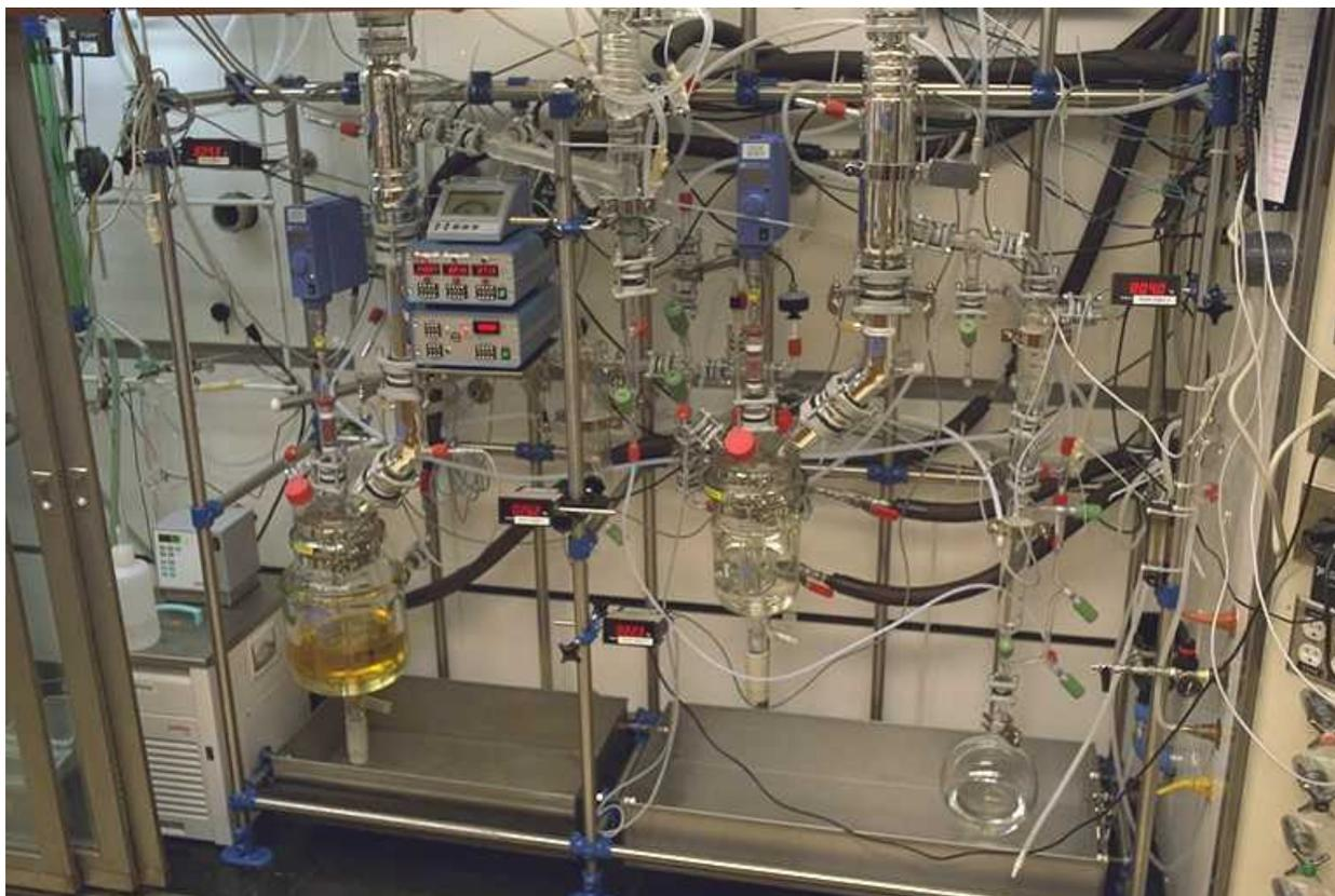
Figure 1. Photograph of the two-reactor system at Roche Colorado Corporation. The 8 liter reactor is at the lower left, and the 5 liter reactor is near the center. Each has a blue IKA stirrer controller above it. The Vacuubrand vacuum controller is on top of the two blue boxes between the stirrers. One Julabo circulator can be seen at the lower left: the others are off the right side of the picture.
