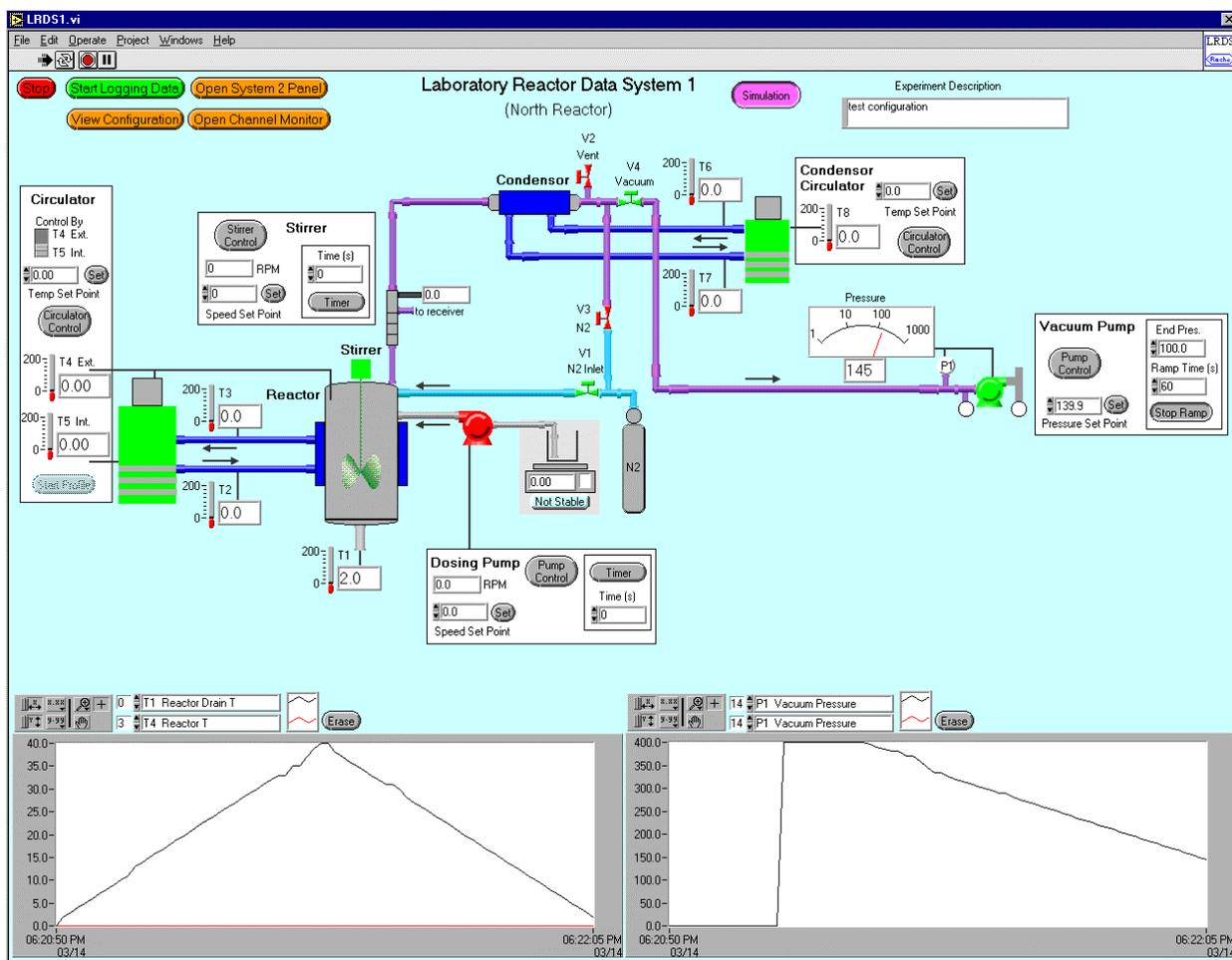
Figure 2. Front panel of the Laboratory Reactor Data System.
