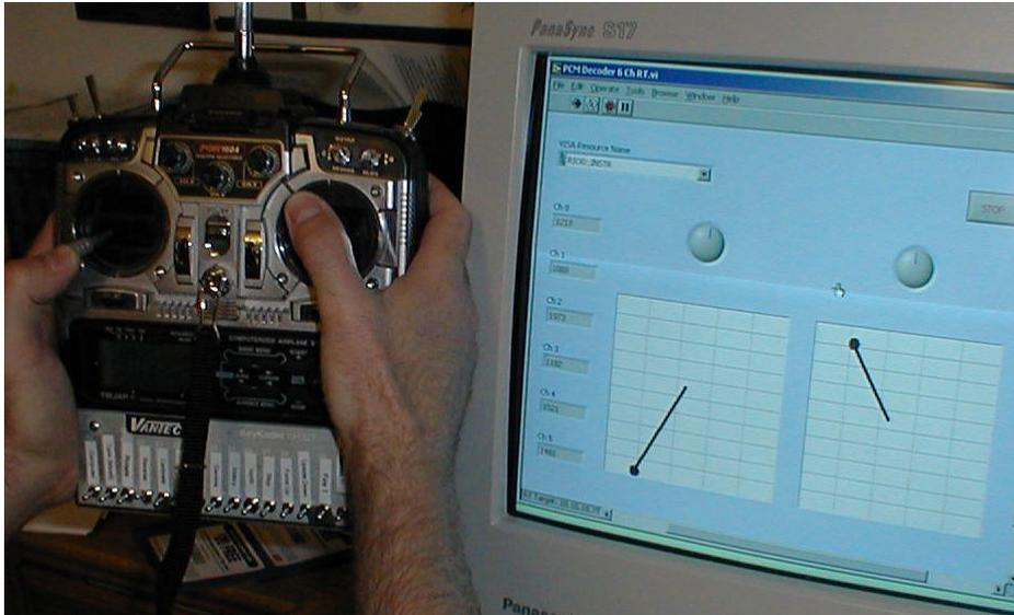
**Figure 3.** Futaba radio being operated by the author while the LabVIEW Real-Time front panel displays the measured joystick positions.
