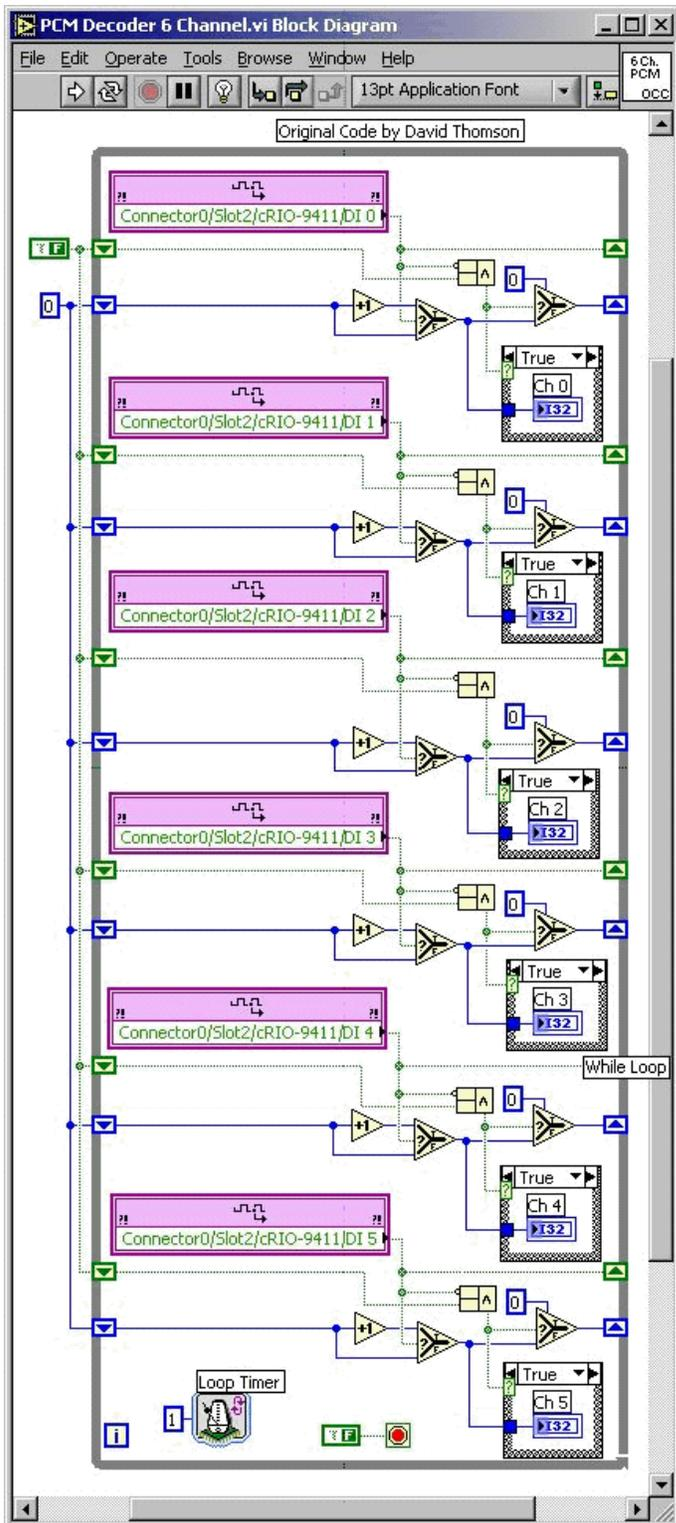
**Figure 1.** The block diagram of the LabVIEW FPGA code for decoding six channels of PCM data using a single 1 microsecond loop and six pairs of shift registers.
