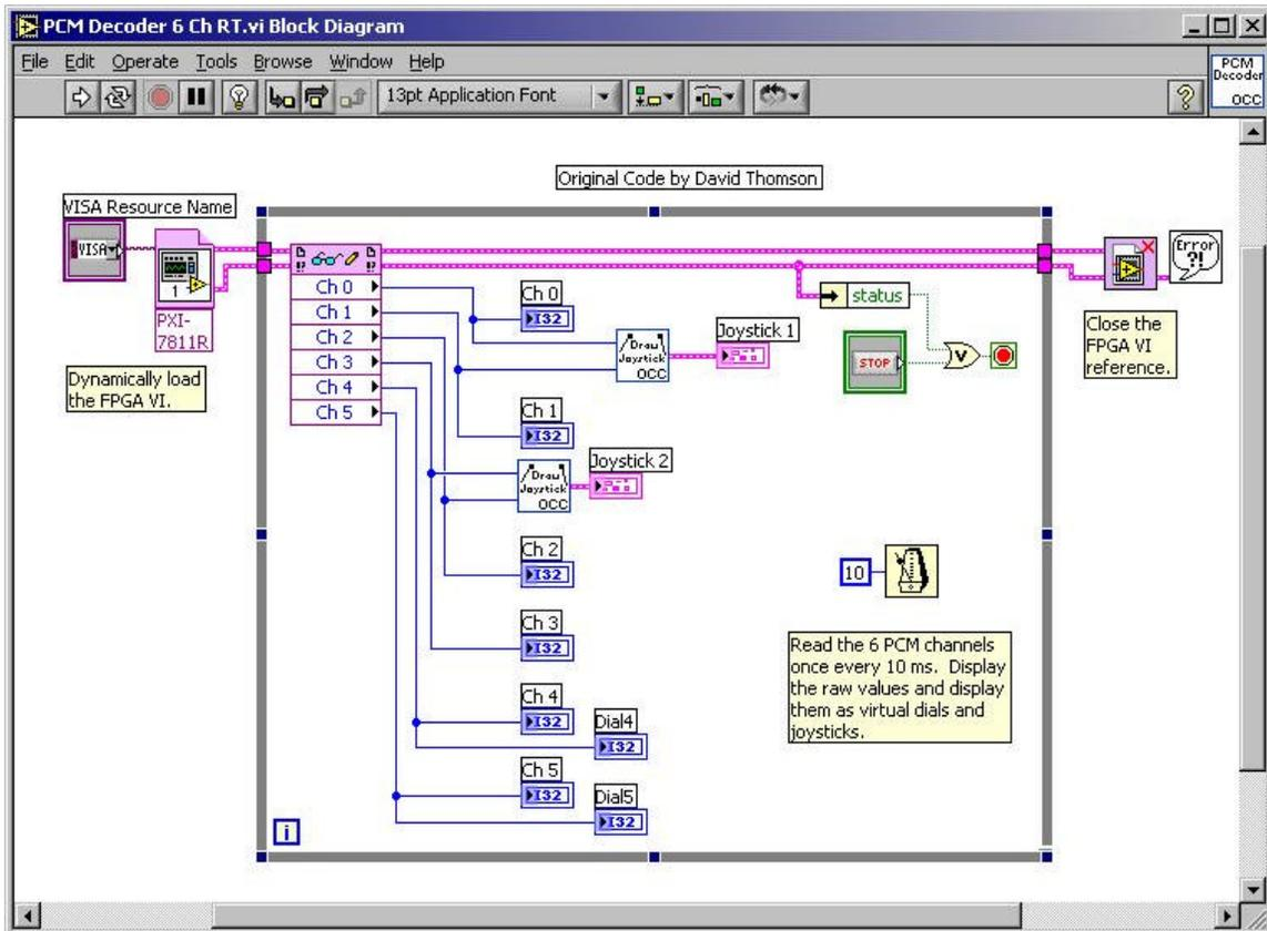
**Figure 2.** Block diagram of the LabVIEW Real-Time code that reads the PCM data from the FPGA. This example VI only displays the PCM data as virtual joysticks and dials, but future versions will apply various control algorithms to this data and then send it back to the FPGA for generation of the calculated control signals.
