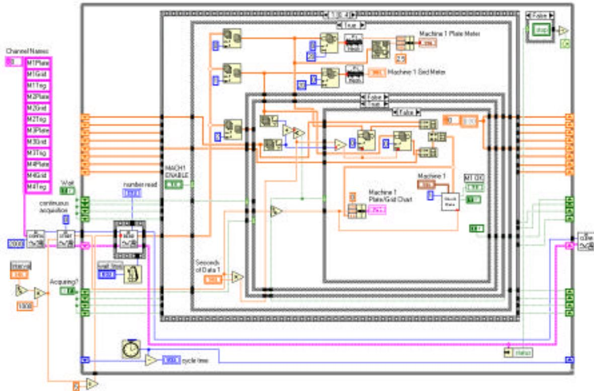
Figure 1. The data acquisition loop. Note that the User Interface loop, which runs in parallel with the data acquisition loop, is not shown. The upper eight shift registers are used to accumulate the two current signals for each of the four machines over numerous loop cycles. The nested case structures control the logic for detecting an event, accumulating the signals, and running the pass/fail algorithm on a complete event.
