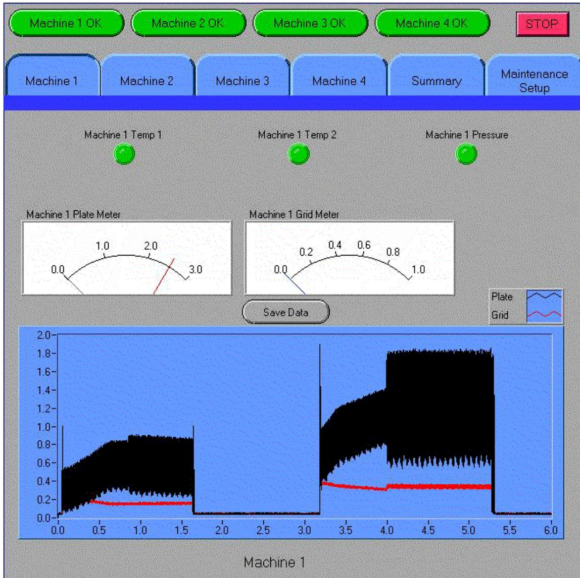
Figure 2. The front panel of the Sealer Monitor program. Pass/Fail indicators for all four machines are always visible at the top of the screen. The row of buttons below those indicators allow the operator to choose which machine to monitor in more detail. Two other buttons bring up a summary of pass/fail results for all machines and a configuration screen.
